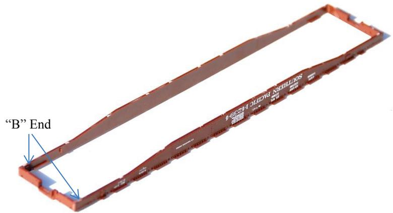
locations while noting the brake lever assembly mounts in the live lever bracket slot and the brake cylinder clevis. Make sure the brake cylinder clevis is pointing towards the “B” end of the car.
